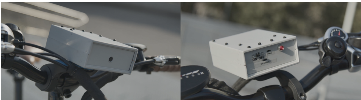
Figure 19. LanePatrol device to collect georeferenced images
