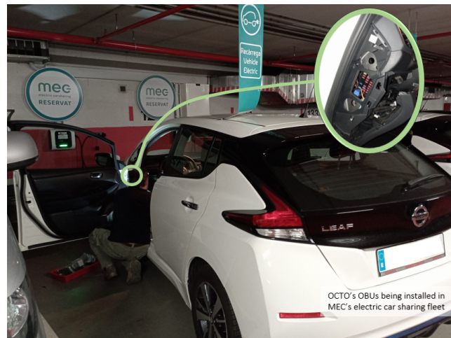
Figure 35. Octo EasyPro being installed in a vehicle from MEC carsharing
